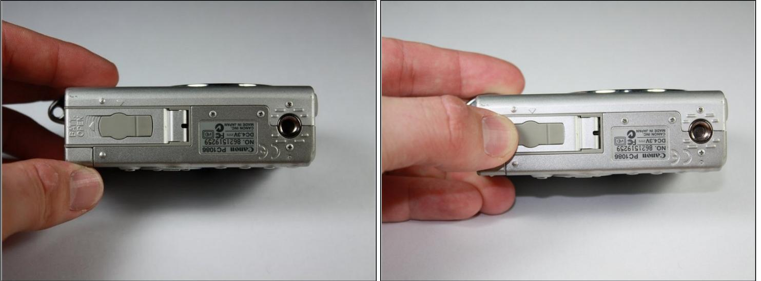
① Turn the camera with the bottom side facing up.
