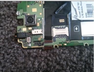
Remove the digitizer cable and separate the digitizer/front glass from the rest of the phone.
