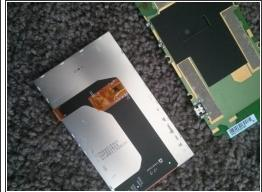
Unplug the LCD screen from the mainboard and carefully peel the display off the mainboard. It is only stuck on.
