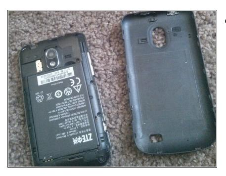
Remove the back cover, SIM card, battery and SD card.
