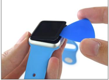
• Heat the screen up so that the entire display and watch are warm. Be sure to turn the device off first by holding down the crown then sliding to power off. Using a sharp blade start at the bottom right corner and lift the glass up enough to create a gap, once you have a large enough gap use a plastic tool to break the adhesive bond around the edges
