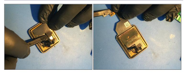
• After desoldering use a plastic spudger in the exact area as the picture shows to loosen up the adhesive holding the digi flex in place. It's best if you use a small amount of heat, around 150F, to help soften the adhesive bond. Fold the digi cable back as shown in the second picture.
