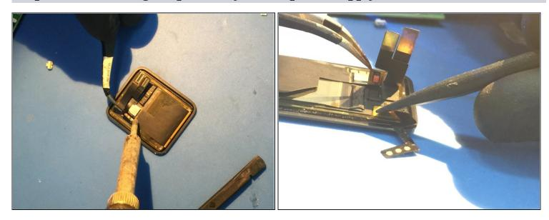
• I used a solder iron tip that was larger than the solder pads. Turn your soldering iron up to a high temperature, 350C is where I kept mine at. DO NOT add any solder, just use the heat & tweezers to pull back the tabs. After unsoldering pull the flex cable out of the way and use tweezers to peel back the proximity sensor from the AMOLED. CAREFULLY.
