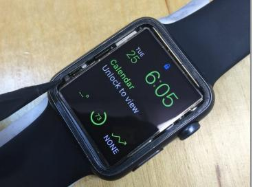
• The AMOLED screen is extremely thin, but not as fragile as you might expect, remember to be gentle and use heat through the entire separation process. To remove the old OCA adhesive use your finger and "roll" the glue off, pure isopropyl alcohol also helps to de-bond the adhesive. The screen is "waterproof" alcohol seeping into the edges is okay.
