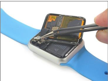
• When inserting the knife & plastic tools around the edges be sure not to go further than 1mm into the AMOLED. The force touch gasket lies directly underneath the glass and is easily damaged if pushed on too hard with a knife or other metal object. The FPC clip is tricky but is easily removed using sharp point tweezers on the battery edge.
