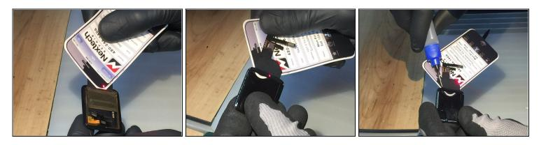
• Begin by preheating the entire screen to a uniform temp, letting it sit under warm air for 10 minutes. I keep my heat gun on 300F-350F while holding the screen 3"-6" away from the nozzle to vary the temperature. Carefully insert a business card under the screen on the dig flex side. Use alcohol to weaken the OCA tape bond then move the card in slow
