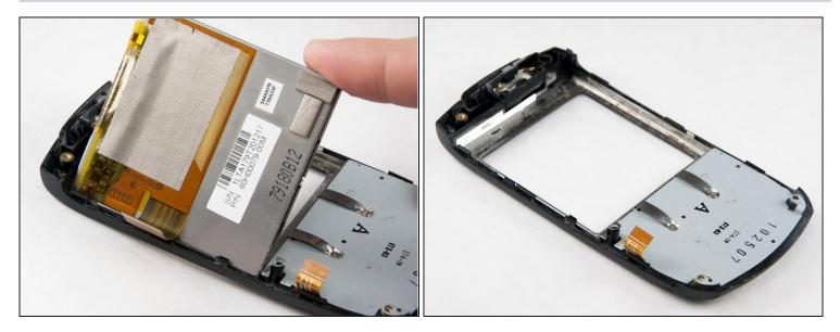
• Using your fingers gently lift the display screen panel out of the casing by either grasping it from the back or popping it out of the front.
