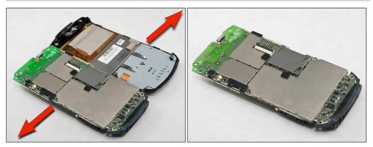
• Separate the circuit board from front cover.
