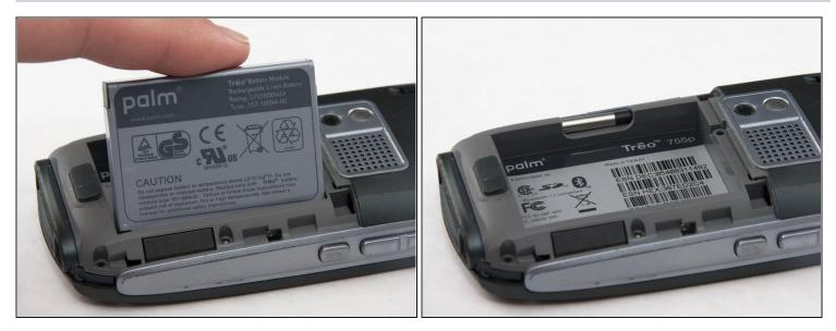
• Remove the battery by lifting up on one side.
