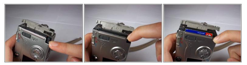
• Push down on the black square button next to the memory card slot. This will release the memory card from the slot.
