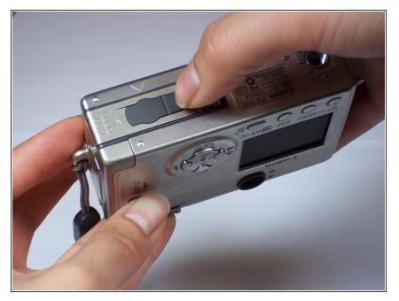
On the bottom of the camera, use your thumb to press the rubber battery cover towards the side of the camera with the strap base. The cover will shift to extend beyond the rest of the camera.
