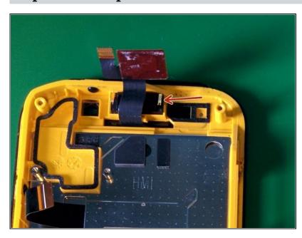
Carefully remove front speaker from the display assembly with spudger tool, can be accessed from indicated side.
