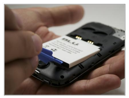
• Using a plastic opening tool or finger, pull out the battery.
