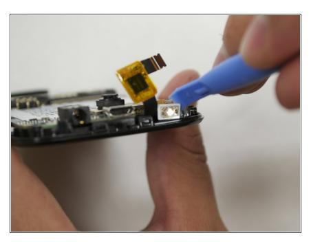
• When the ribbon cable is removed from the ZIF connector, peel off the power sticky button using a plastic opening tool.
