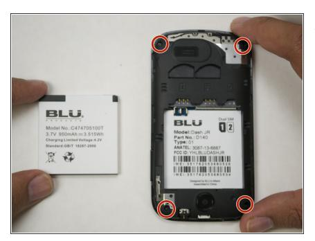
Remove the four 4.0mm Phillips #1 screws.
