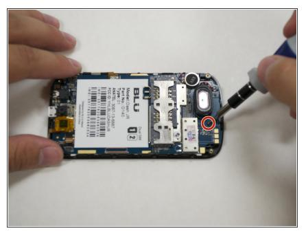
• Unscrew the 3.6mm Phillips #0 screw from the motherboard.
