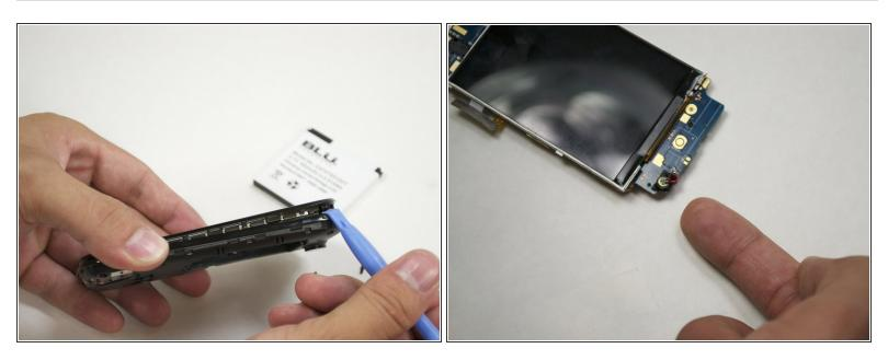
Starting from a corner, separate the panel from the frame using the plastic opening tool.
