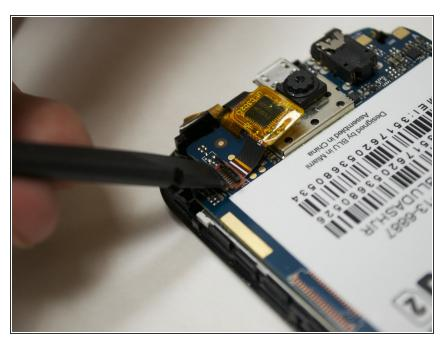
• Using a spudger, lift the black ZIF connector at the top left corner of the phone.
