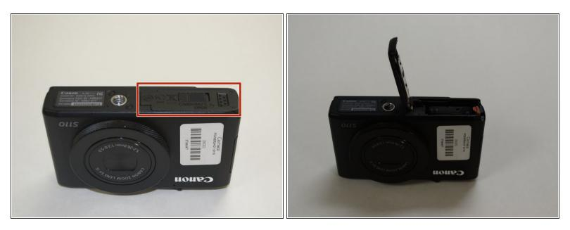
• Remove the battery by sliding open the cover on the bottom of the camera.
