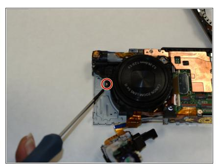
• Remove the Phillips screw on the front facing side of the lens.
