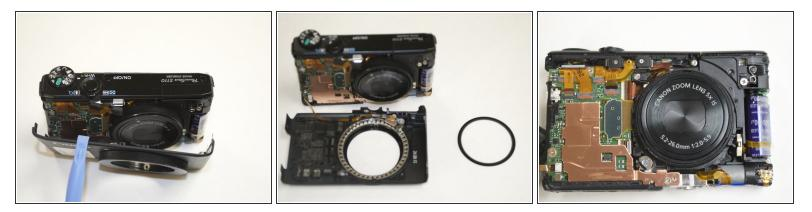
• In order to remove the other two connectors, the front of the case must be removed. Slowly pry around the edges using a plastic prying tool to free the case. A lens-ring piece will fall out from the inside of the camera; set this aside.
