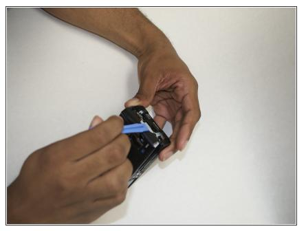
• Release all clips around the outside plastic shell, and it will lift off.
