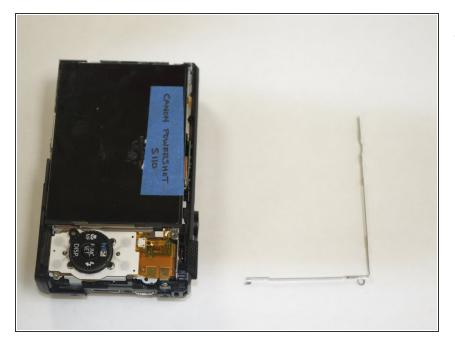
• Lift out the display mounting bracket, and set it aside.
