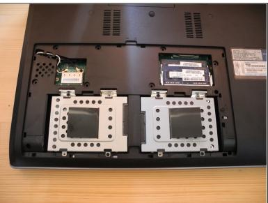
Gently slide your new SSD/HDD in the empty HDD bay. And do not forget to secure it to the body of the laptop with a few screws.
