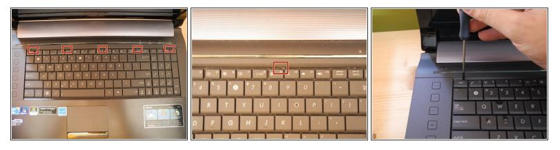
Use a small flathead screwdriver or the flat end of a spudger to gently push down the five pins just above the top row of keys that secure the keyboard to the laptop.
