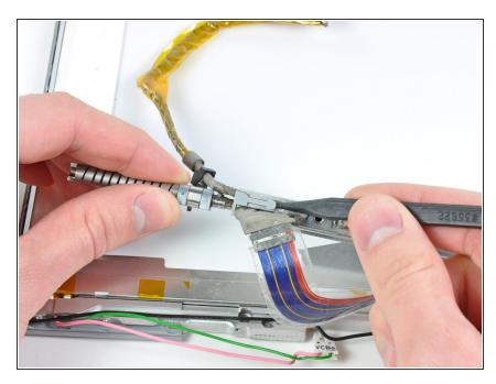
Use the tip of a spudger to remove the gray plastic end cap from the display data cable side of the clutch hinges.
