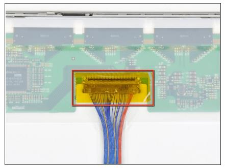
i If present, remove the strip of tape covering the display data cable connector.
