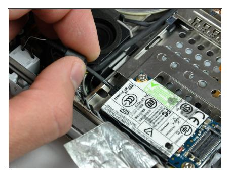
Disconnect the RJ-11 cable from the modem.
