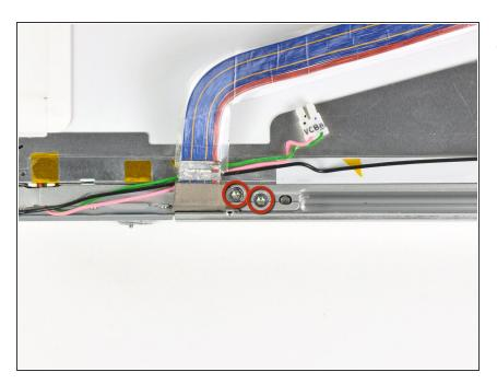
Remove the two 10.3 mm T8 Torx screws securing the clutch hinges near the display data cable.
