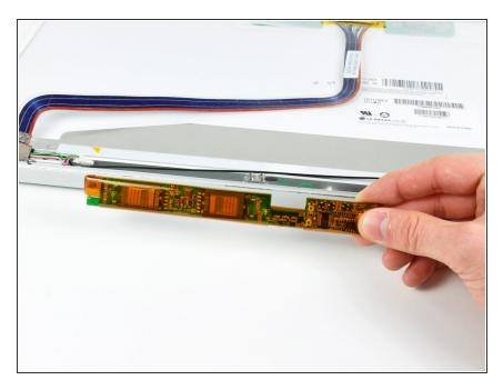
Remove the inverter from the display.
