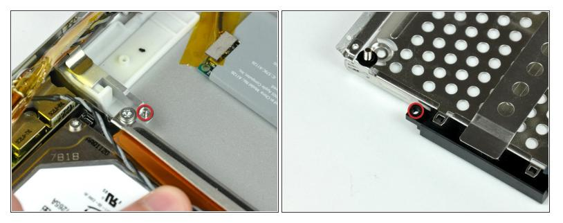
When reinstalling your PC card cage, be sure to insert the post sticking up from the PC card release button into the hole in the black plastic release mechanism on the PC card cage.
