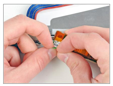
Disconnect the backlight cable from its socket on the display inverter.
