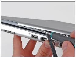
• Insert the flat end of a spudger between the rear display bezel and the plastic rim attached to the front display bezel near the lower right corner of the display.
