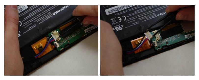
Using needle-nose tweezers, gently push the large white wire connector (connected to the black, red and blue wires) out of its housing.
