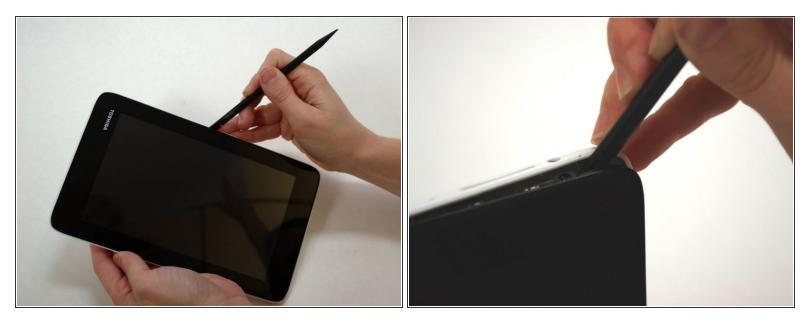
(i) To replace the battery, the rear cover must first be removed.
