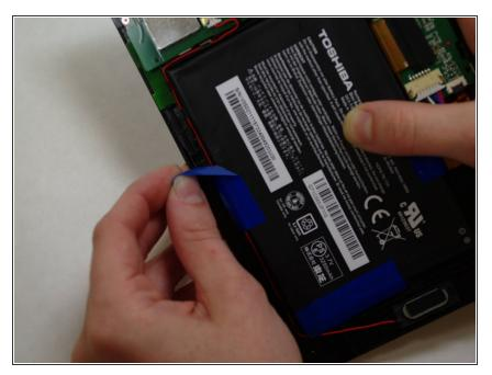
• Carefully remove the electrical tape that holds the battery in place.
