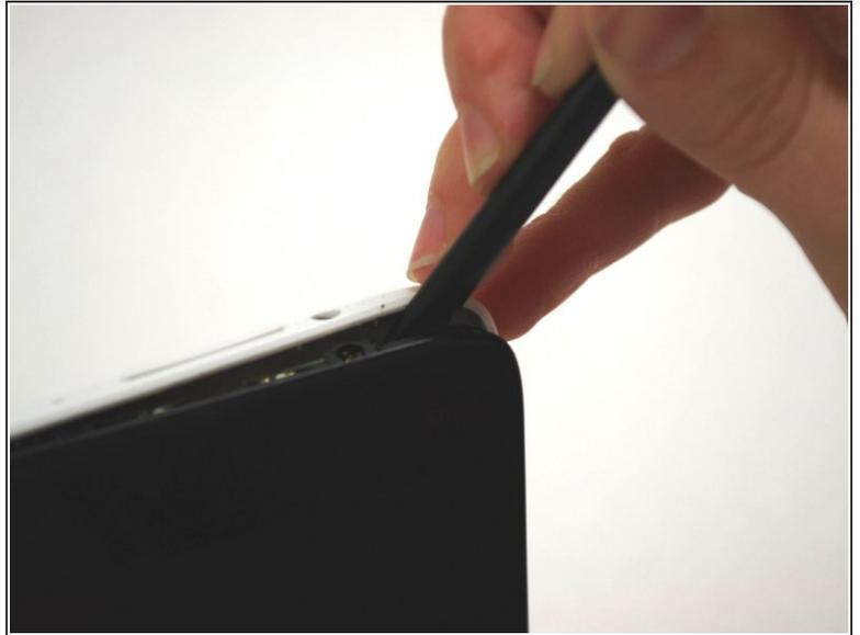
***i*** To replace the battery, the rear cover must first be removed.
