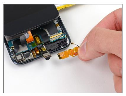
• Remove the Wi-Fi antenna from the iPod Touch.
