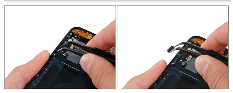
• Use tweezers to remove the volume-down button from the iPod.
