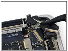
• Remove the rubber hinge covers from the right and left display hinges.
