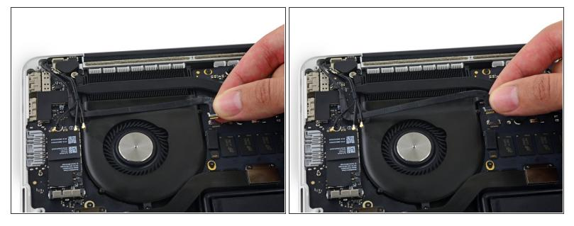
Peel the iSight camera cable up off the fan housing.
