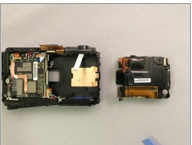
Using the plastic prying tool, pry the lens box from the camera.
