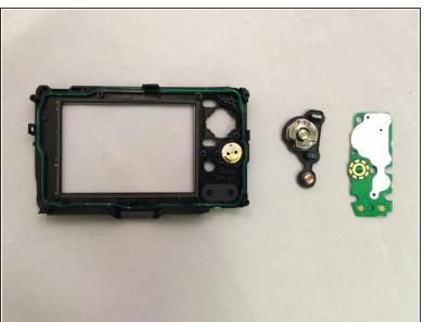
Use your fingers to lift the green circuit board and buttons out of the case.
