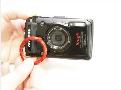
Remove the red ring surrounding the lens by twisting it counter-clockwise
