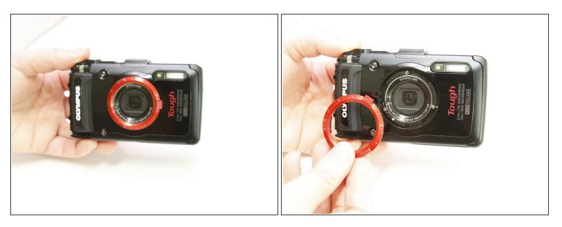
• Remove the red ring surrounding the lens by twisting it counter-clockwise
