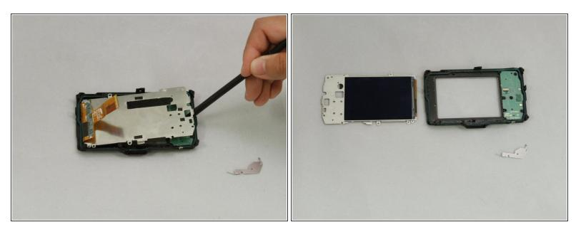
Using the spudger on the edge of the screen to lift it and remove the metal backing attached to the screen.
