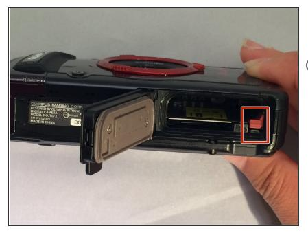
Press the red tab to eject the battery.
