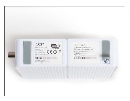
Lift rubber feet and reveal the two Torx 10 screws.
