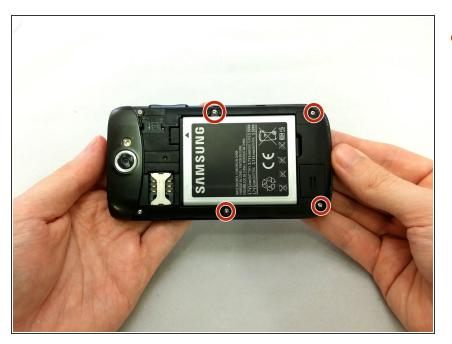
Remove the four 3.8mm Phillips #000 screws securing the back assembly to the phone.
