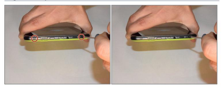
• There are two screws on the side with the micro USB power port. Remove the two 2mm x 0.5mm screws with a Phillips #0 Screwdriver head.
