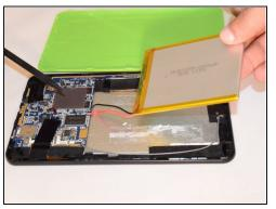
• 4. Remove the tape holding the battery to the plastic frame. The battery is glued to the back of the LED. Pry the battery off the LED using a <u>plastic card</u>.
