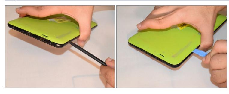
Pry off the plastic backing with the spudger and the plastic opening tools. Anything that can provide enough leverage and not conduct electricity will also work for this purpose.
