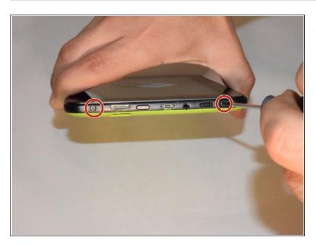
There are two screws on the side with the micro USB power port.
