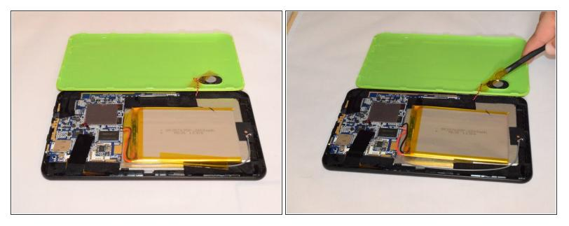
Once you pry off the plastic backing, you will expose the battery and the motherboard. Then
