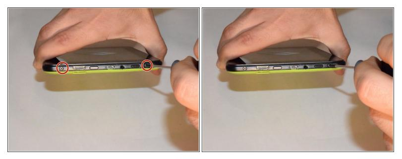
There are two screws on the side with the micro USB power port. Remove the two 2mm x 0.5mm screws with a Phillips #0 Screwdriver head.
