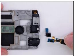
Use the flat end of the spudger to remove headphone jack component from rectangular housing.
