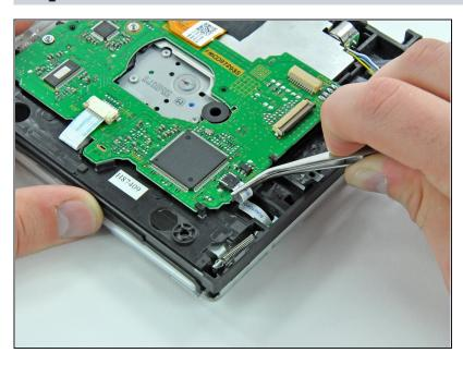
Pull the disc detector ribbon cable straight out of its connector with a pair of tweezers.
