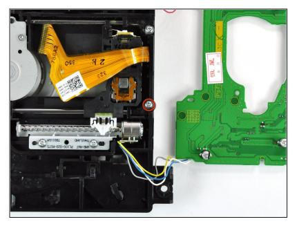
Remove the 5.0 mm Phillips screw that is closer to the yellow, blue, white, and grey wires.
