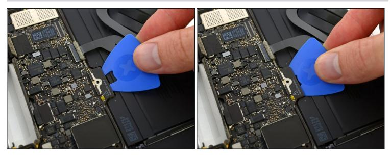
• As an added precaution, you may physically disconnect the battery by inserting a <u>battery isolation pick</u> between the logic board and the battery connector.
