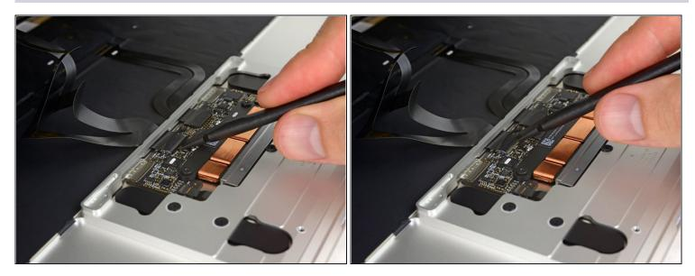
• Use a spudger to carefully flip up the retaining flap on the trackpad cable ZIF connector.
