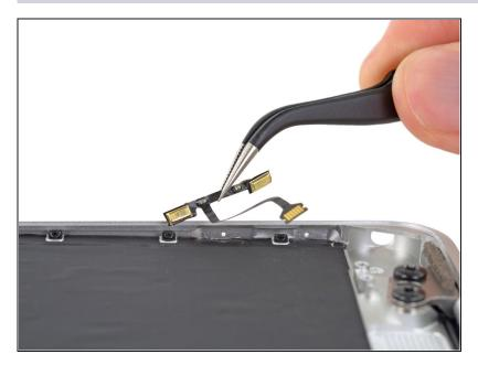
• Remove the dual microphone assembly.
