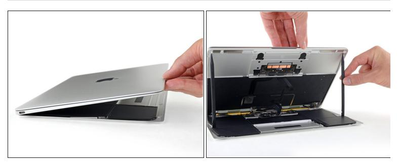
• Lift the upper case and display together from the front edge and raise it to about a 45° angle.
