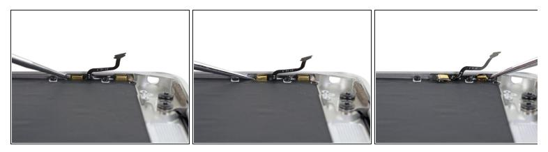
• Use a fine-tip probe or pick to gently peel the dual microphone assembly away from the case.
