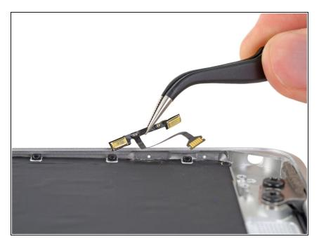
• Remove the dual microphone assembly.
