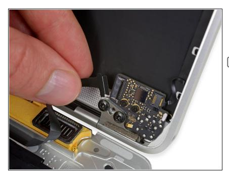
• Disconnect the audio jack board ribbon cable by pulling it straight back out of the ZIF connector.
