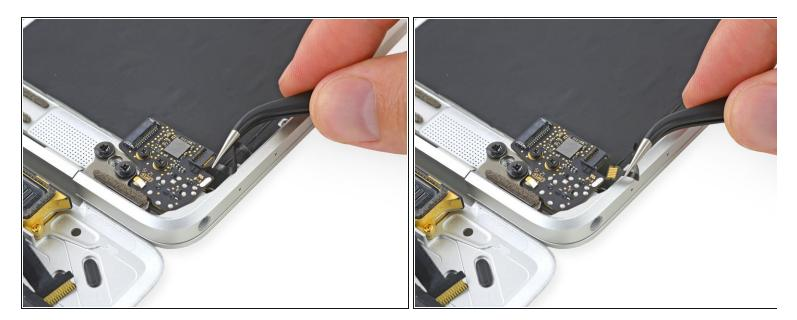
• Disconnect the microphone assembly ribbon cable by pulling it straight out of its connector.
