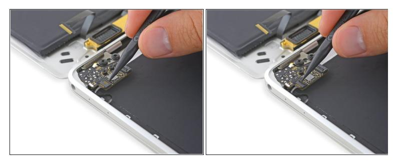
• Use a spudger to flip open the ZIF connector retaining flap for the dual microphone assembly ribbon cable.
