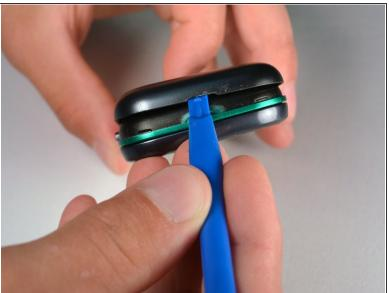
Pry the back cover off with a plastic opening tool, or your fingernail, in the indentation on the bottom of the device.
