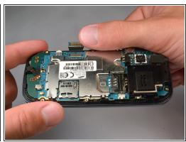
Use your finger nail to disconnect the display data cable from the motherboard.
