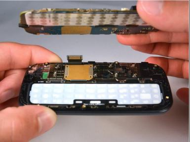
• Carefully lift the main motherboard assembly away from the front panel.
