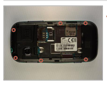
Remove the six 3 mm #00 Phillips screws in the plastic back frame.
