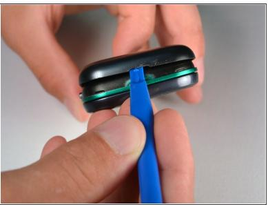
Pry the back cover off with a plastic opening tool, or your fingernail, in the indentation on the bottom of the device.
