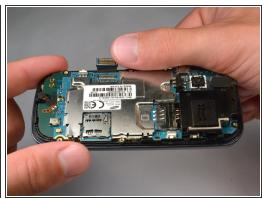
Use your finger nail to disconnect the display data cable from the motherboard.
