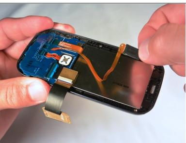
Use a spudger to get underneath and remove the call speaker.
