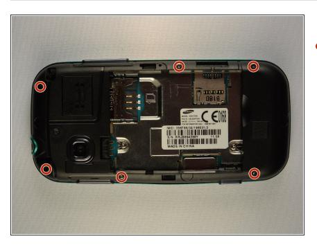
Remove the six 3 mm #00 Phillips screws in the plastic back frame.
