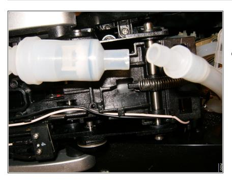
Test the check valve. Blowing air in it from the boiler side should cause it to open. Repeat that a couple of times to loosen any sediments etc. It will also help to run some hot water from the K-cup side into the check valve and shake it up. Once it is cleaned, replace the check valve and the tie straps. Reassemble the Keurig To reassemble your device, follow these instructions in reverse order.
