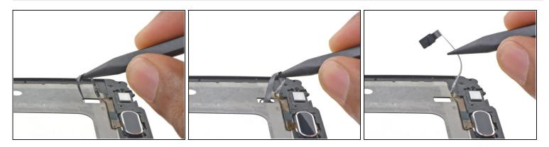
Flip the display frame over and use the pointed end of a spudger to pull the home button cable completely through the hole.
