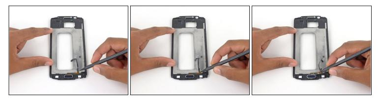
Slide the spudger under the cable to continue separating it from the frame.
