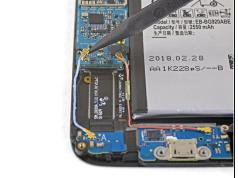
Use the pointed edge of a spudger to disconnect the Bluetooth and Wi-Fi antenna cable connectors from their sockets on the motherboard.
