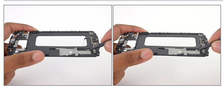
• Use the pointed end of a spudger to push the home button cable through the display frame.
