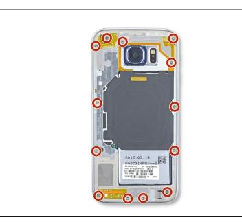
• Remove the thirteen 3.5mm Phillips #00 screws securing the midframe to the phone.
