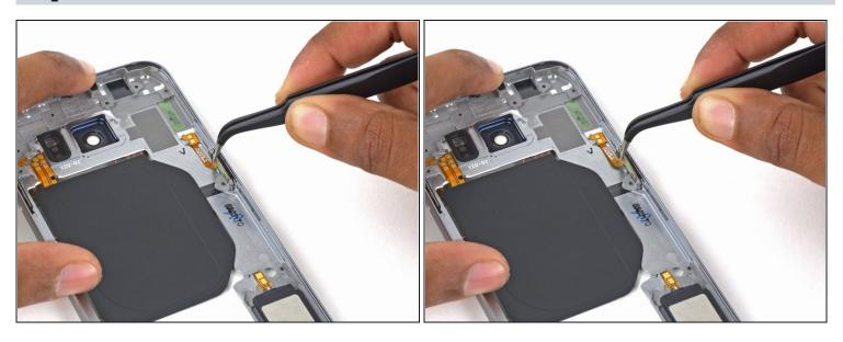
• Using the angled <u>tweezers</u>, grip the power button bracket and pull it out of its socket.
