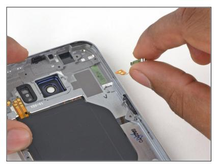
• Remove the power button bracket assembly.
