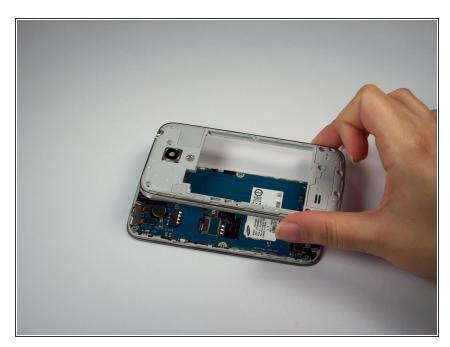
Using the <u>USB board replacement</u> guide, step 3 - 8 in reverse order to place the back cover, making sure the wires to the charging pad fits through the ready made holes.
