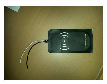
Soldering on thin flexible wires to the + and - on the wireless charging pad
