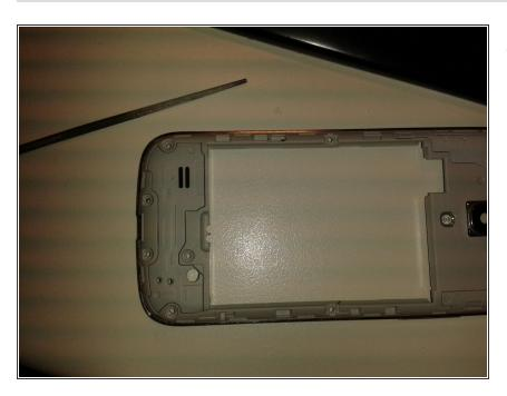
Use a small file to make room for the wires on the back frame just below where the battery sits.
