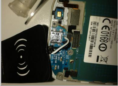
Soldering the wireless charging pad connection + to CN2 on the USB port and - to the ground on the USB port, any part of the external metal surface should work.
