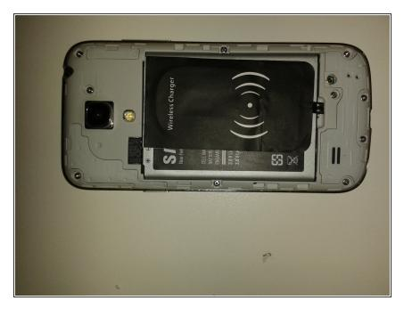
Placing the wireless charging pad, slightly off center to keep NFC, which is implemented in the battery, working.
