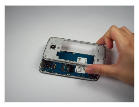
Start by using the <u>USB board</u> replacement guide, step 1 - 8 in order to gain access to the USB board.
