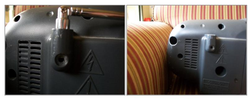
• Remove 1 screw to remove the antena.
