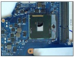
Use the same technic to clean the surface of the processor from the old thermal compound.
