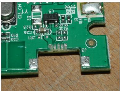
A broken off micro-USB connector for charging a bluetooth keyboard doesn't seem like a challenge. But wait until you've tried with this one: Rapoo E6700 bluetooth keyboard.
