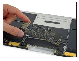
• Remove the logic board.
