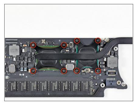
Remove the eight 2.5 mm T5 Torx screws securing the heat sink to the logic board.
