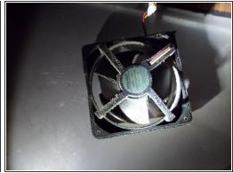
• The fan has a white Bracket with some foam at a gaspipe. I have no Photo of that part, but you can see it in Step #9. Goto to #9, Ja. ...carefully remove it. There is a plug with a clip. The fan has no screws and no clipse. Just pull it carefully. Very easy!
