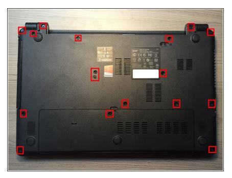
Remove 17x Philips screws
