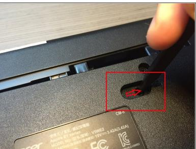
Press and slide battery-lock button to remove the battery.
