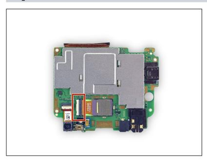
Following the procedure from steps 19 & 20, open and disconnect the ZIF cable close to the center of the circuit board.
