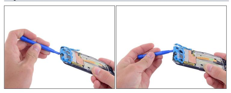
• Using a plastic opening tool, lift the turquoise case from the end near the headphone jack.
