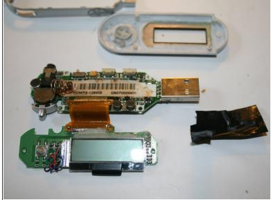
Remove casing and remove plastic protection.
