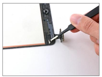
i If necessary, use a pair of tweezers to partially peel back the piece of tape covering the smart cover magnet near the lower left corner of the front panel assembly.
