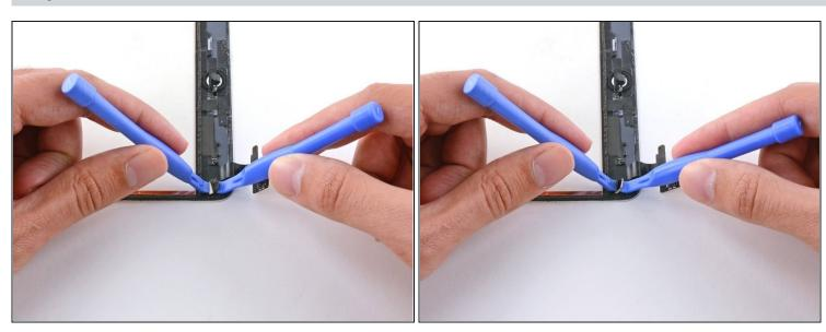
Use the previously described procedure to remove the smart cover magnet near the bottom left corner of the front panel assembly.
