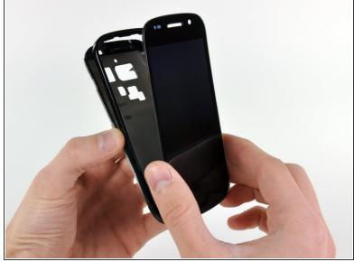
Removing the display presented us with the first stumbling block in our disassembly. A heat gun made quick work of the front case assembly, though.
