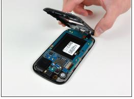
After removing six screws with our trusty Phillips #00 screwdriver, a little prying with a plastic opening tool lets us remove the inner case.
