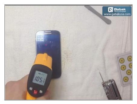
a peak of 105 degrees is fine but keep it moving fast the gun so the heat will spread even in the whole LCD
