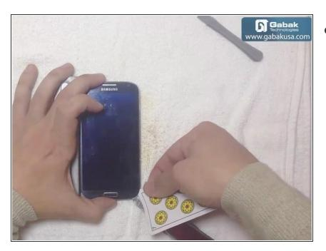
lift the glass with the blade and put the card
